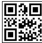
Fig. 1. Exemplary 2D barcode having three positioning elements (markers)
